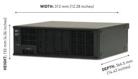
Height: 103 mm (4.062 inches) Width: 312 mm (12.28 inches) Depth (w/cable cover): 366.5 mm (14.43 inches) (w/o cable cover): 303 mm (11.93 inches) Weight: approx. 5 kg (approx. 11 lbs)
