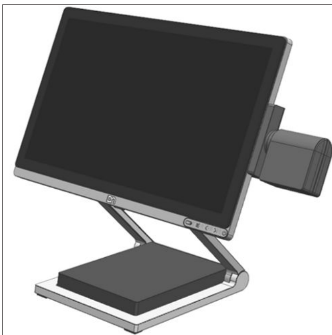
Figure 10-26: System overview with BCR
