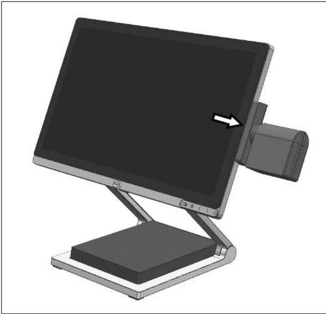
Figure 10-36: Snapping back the BCR top cover
