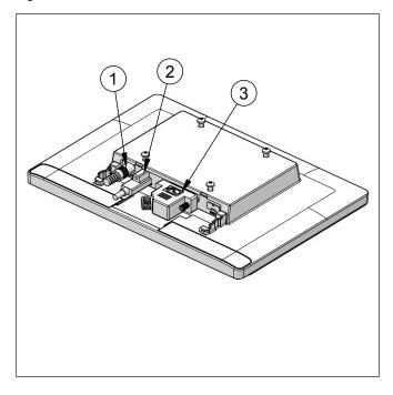
Figure 8-6: Attaching all cables to the display
