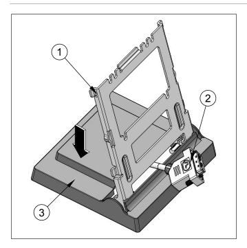
Figure 8-4: Manage cabling through the lower back cover
