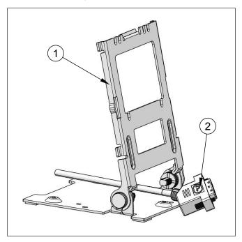
Figure 8-3: Manage cabling through the stand
