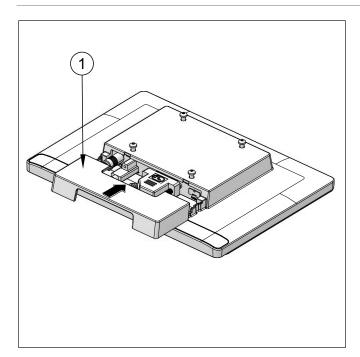
Figure 8-7: Mounting the cable cover
