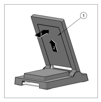
Figure 8-1: Removing the upper back cover
