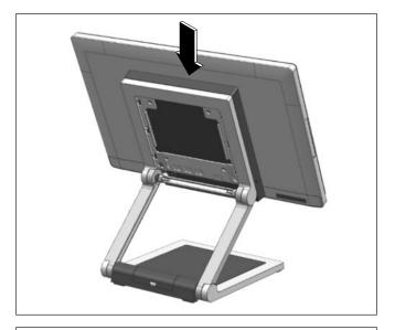
1. Fit the system on the stand while holding it in place.
