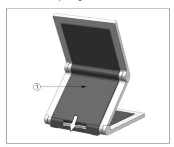
1. Remove the back cable cover (1) by sliding it downwards (indicated by arrow).
