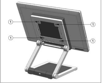
2. Tighten the 4 M4x6 countersunk screws (1) (that came with the stand) to secure the system to the stand.
