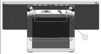
5. Plug the USB-C cable into the port indicated (1).
