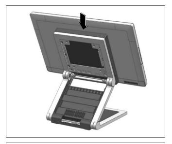
1. Fit the system on the stand while holding it in place.
