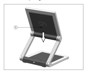
Remove the VESA cover by sliding it downwards (indicated by arrow).
