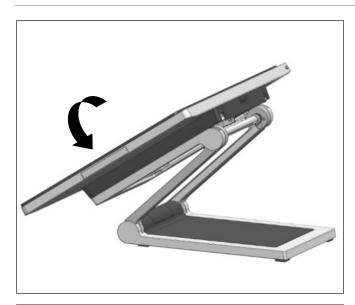
3. Tilt the system back to access the connector panel at the bottom of the system display.
