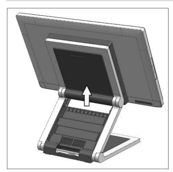
10. Replace the VESA cover by sliding it upwards.
